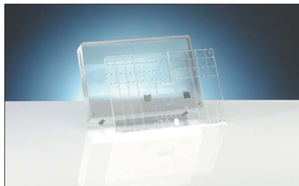
Test phantom for quality control of analog mammographic X-ray installations
